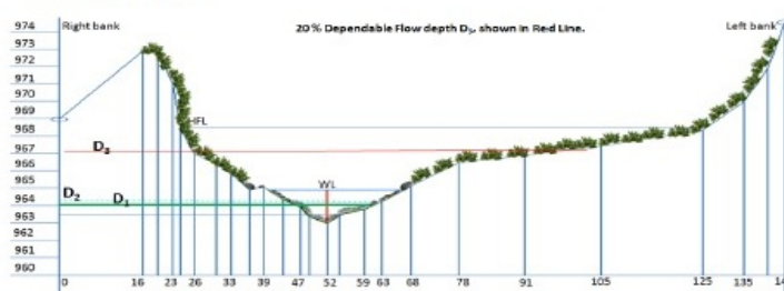
Figure 5.5: River Cross-section at Ranari, Dharasu
